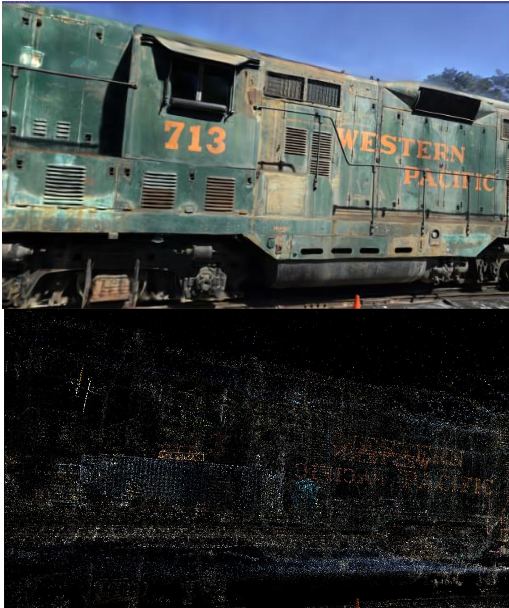
Figure 5: Top: Shows the rendered outputs of the system with the gaussian splats set to 1 (full size). Bottom: shows the rendered outputs of the system with the gaussian splats set to minimum size to show the point cloud.
