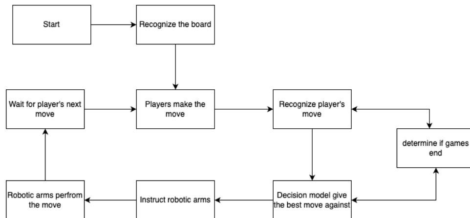
The Chinese Checkers-playing robot operates in a structured loop that begins with setting up the board and continues through the game until a win condition is reached.
