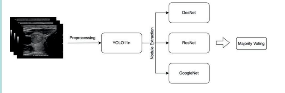
The system processes ultrasound examination data, either as a video or a sequence of consecutive images. A YOLO-based detection model identifies thyroid nodules in each frame, generating bounding boxes that define regions of interest (ROIs). These ROIs are extracted and passed to a classification model for analysis.
