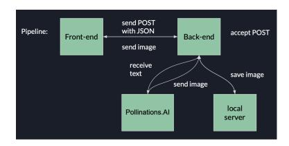
The overall pipeline of the feature is shown in the above flowchart. The user could send a post request with the input vocabulary as the body to the backend server. Then, the backend server will communicate with the pollination AI to get the image that corresponds to the vocabulary. The image will be saved on the local server. After that, the image will be sent back to the user front so that the user can observe the image corresponding to the vocabulary.
