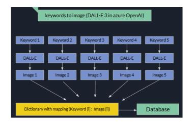
Once keywords are extracted, the system iteratively generates corresponding images. Each keyword is passed to DALL-E 3, which produces a representative image. This keyword-image pair is then stored in the database. This process repeats until images have been generated for all extracted keywords. The database then serves as the source for the frontend, providing the necessary data to create the flashcards.
