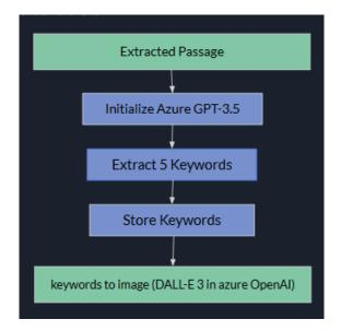
This service accurately converts the input JPEG image containing the text passage into a text string. This extracted text is then fed to Azure GPT-3.5 for keyword extraction. A carefully crafted prompt guides GPT-3.5 to identify a specified number of relevant keywords, ensuring they are non-violent, distinct, and feature complex character strokes suitable for SEN student recognition.
