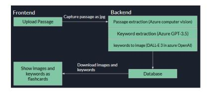
The JPEG passage is passed to Azure Computer Vision for recognizing the passage outputted as a text string, which is passed to the keyword extraction function to extract keywords using Azure GPT-3.5 (with the number of keywords depending on the prompt). Each keyword is drawn to generate the corresponding image, and the keyword-to-image mapping is then into the database, which will be extracted by the front end to make flashcards with the corresponding keywords and images.
